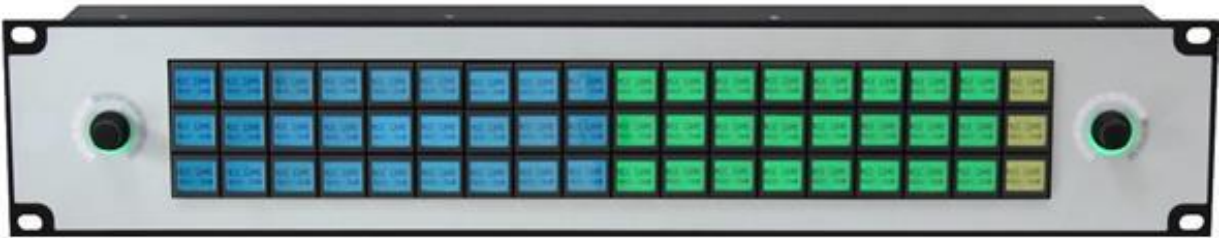
MTOUCH-PUSH54 - 19" 2RU MAGELLAN TOUCH PANEL WITH 54 LCD PUSH BUTTONS, 2 ROTARY ENCODERS
