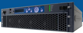
This multichannel uncompressed-over-IP module provides uncompressed signal transmission at high bitrates and quality for superior editable video, and is especially well-suited to low-latency broadcast contribution applications such as sports, live events and studio-to-studio production. Supporting real-time transport of \*3G/HD/SD and IP, this card enables high-density, multichannel uncompressed over IP in a single-slot solution that provides up to 112 UCIP channels in the Selenio MCP3 platform.
