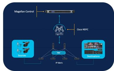
Routing operations are performed in parallel on "A" and "B" networks in 2022-7 hitless configurations – for full 1+1 redundancy along the way from end to end.
