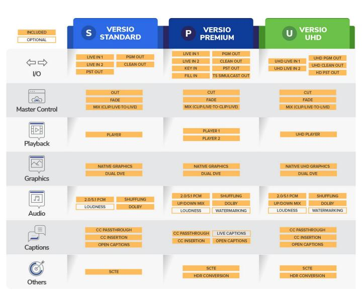
NOTE: Versio Premium Channels – Key/Fill not supported with transport streams, HDR conversion not supported with SDI, TS Simulcast only available with SDI or ST 2110
