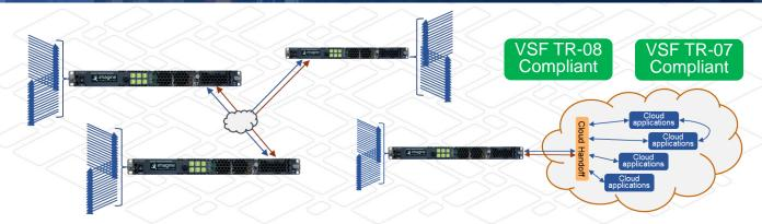
Selenio™ Network Processor (SNP) is a high-density, scalable, reconfigurable platform that enables media companies to perform video processing and conversion functions on standards-based IP networks using the SMPTE ST 2022-6 and ST 2110 standards, while also supporting SDI and Typical applications 12G-SDI. include connecting between facilities or transporting signals to/from cloud-hosted applications.
